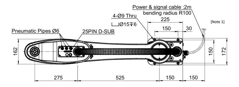
[Note 1] Cable bending radius of at least 150mm, please reserve space to deploy the cable
