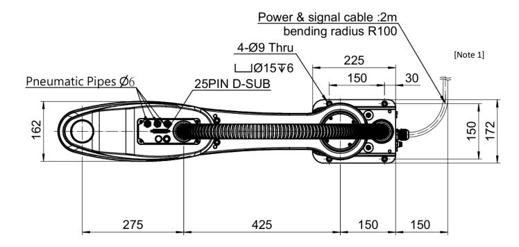
[Note 1] Cable bending radius of at least 150mm, please reserve space to deploy the cable
