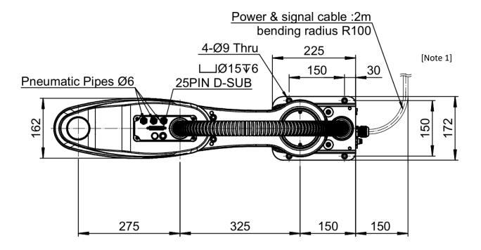
[Note 1] Cable bending radius of at least 150mm, please reserve space to deploy the cable
