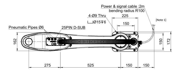
[Note 1] Cable bending radius of at least 150mm, please reserve space to deploy the cable
