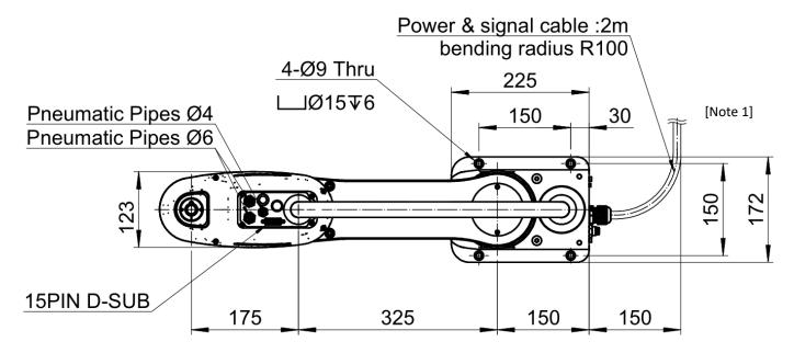
[Note 1] Cable bending radius of at least 150mm, please reserve space to deploy the cable
