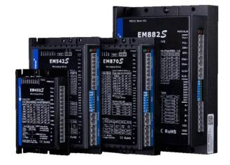
heating & noise. All the micro step and output current configurations can be easily done via built in DIP switches. Its control type (step & direction or CW/CCW) and command smooth filtering can also be configured via DIP switches. Therefore, the EM series is an ideal choice for many applications requiring simple step & direction or CW/CCW control of NEMA 17, 23, and 24 stepper motors.
