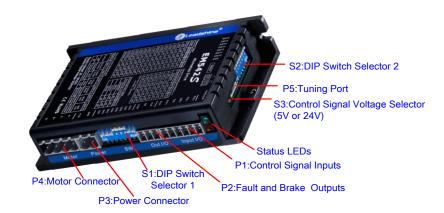
The EM series has 5 connectors P1, P2, P3, P4 and P5, 3 DIP switches S1, S2 and S3. P1 is for control signal connections, P2 is for fault output, P3 is for power connection, P4 is for motor connection and P5 is for fine tuning. **Note: This segment is not available for EM522-CAN and EM556-CAN.**
