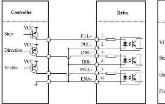
Figure 1 Connections to open-collector signals (Common-anode)
