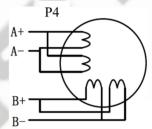
Figure 12 8-lead motor parallel connection
