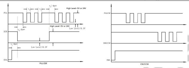
Figure 13 Sequence chart of control signals
