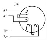
Figure 11 8-lead motor series connection
