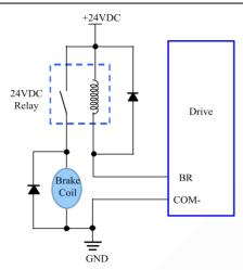
Figure 7 Brake Output Connection
